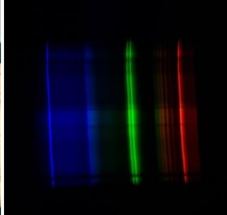
Light emission Spectrum of a low-consumption light bulb (cold light) obtained with the mobile transformed into a spectrophotometer.
