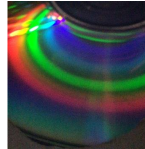
Light emission Spectrum of a low- energy light bulb (warm light) obtained with the Mòvil transformed into a spectrophotometer
